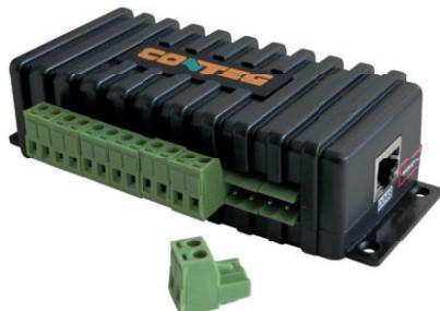
The expander allows creating 8 inputs/outputs on a single smart port of the main control and monitoring unit. The expander's input contact is capable of supporting any type of door contact (e.g. RMS-MK-01). The device is automatically recognized and powered from the main unit. The expander is connected using a standard LAN CAT 5/6 cable. Maximum cable extension length is 300 m.
