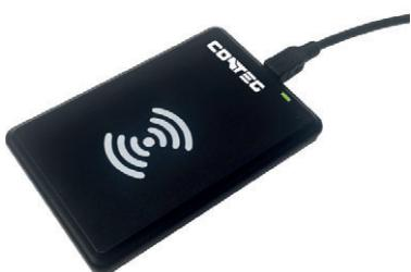
This desktop dual card reader for PC is a handy peripheral for user card administration in the CONTEG Pro Server application. The reader operates on 125 kHz and 13.56 MHz frequency. It is capable of working with 125 kHz identification media for access control and is fitted with LED signalization and a buzzer. The reader connects to the computer's USB port, from which it also draws power.
