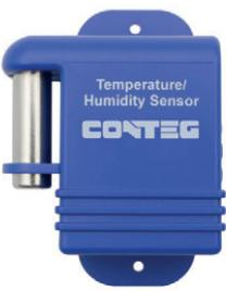
The encased temperature and humidity sensor is designed for placement inside racks and measures temperature in -55 °C to +75 °C range and humidity in 0 – 100 % range. The sensor can be extended for reach of up to 300 m using a LAN CAT 5/6 cable.
