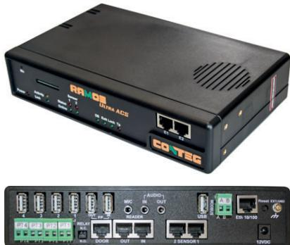
The RAMOS ULTRA ACS main control and monitoring unit monitors up to 50 racks via rack door units (RDUs) which are connected in a daisy chain to 2 expansion ports. In addition, the use of RAMOS ULTRA-EX-I8 expansion module allows the control unit to monitor up to 500 sensors.
