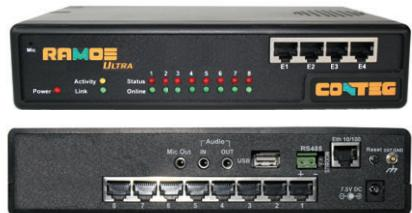
The RAMOS ULTRA main control and monitoring unit monitors up to 100 racks via rack door units (RDUs) which are connected in a daisy chain to 4 expansion ports. In addition, the use of RAMOS ULTRA-EX-I8 expansion module allows the control unit to monitor up to 500 sensors.
