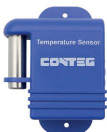
The temperature sensor is designed for placement inside racks and measures temperature in -55 °C to +75 °C range. Up to 8 sensors can be chain linked to a single smart port. The sensor is powered from the main unit. Extension is done using a standard LAN CAT 5/6 cable. Maximum cable extension length is 150 m for 8 sensors.
