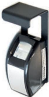
This extremely durable, high-performance optical fingerprint reader boasts a scanning resolution of 500 dpi/8 FPS and scanning area size of 13 × 16 mm (256 × 320 pixels). The reader is adapted for maximum communication distance of 5 m. Powered from the main unit.
