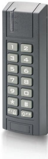
Backlit keypad with built-in card reader (EM format) enables authentication either using only a card on the 125 kHz frequency band, or using a combination of a card along with a four-character code. Easy connection to an RDU via a cable with color-coded RJ-45 connector. The reader is equipped with a buzzer and status indication LEDs. Suitable for installation in indoor areas. Low power consumption of only 65 mA in standard operation. Powered from the main unit.
