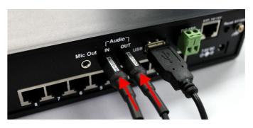
d) Now you will connect the opposite end of the audio cable into the audio jack on the USB modem as shown above. The picture also shows where you would insert your local service provided GSM SIM card.
