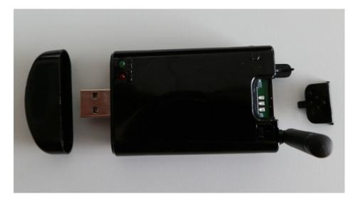
To install the EDGE-180M USB as a modem, please plug in EDGE-180M USB modem to USB port on the back of the unit using the USB extension cable provided with the modem.
