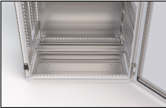
50 mm space from the ground to the bottom edge of the door allows for installation without the need of additional plinth, thanks to a specially designed bottom frame. This solution does not reduce the space for internal installation.
